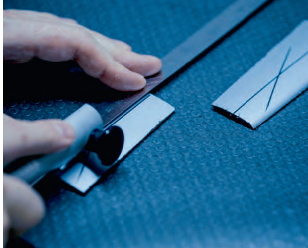
Left image: Zelfl uses a special tool to cut the material sample prior to the pressurized water test (right).
