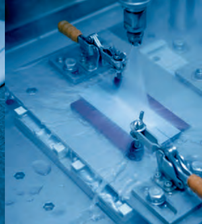
Left image: Zelfl uses a special tool to cut the material sample prior to the pressurized water test (right).
