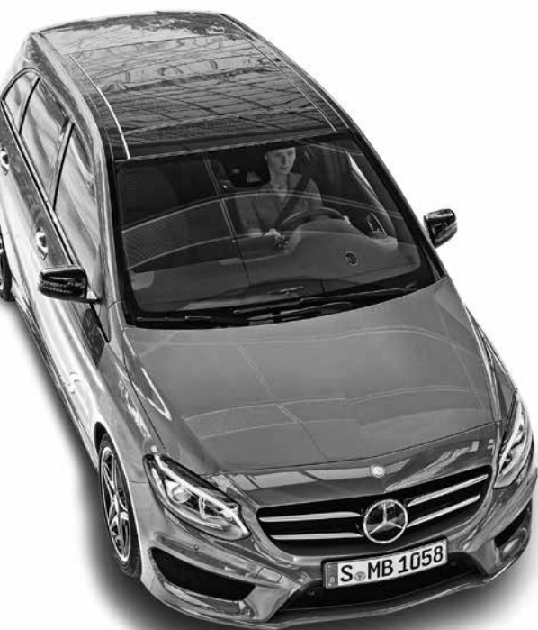
Stick-on paints: the water deflector on the Mercedes B-class are painted with film from Wörwag.
