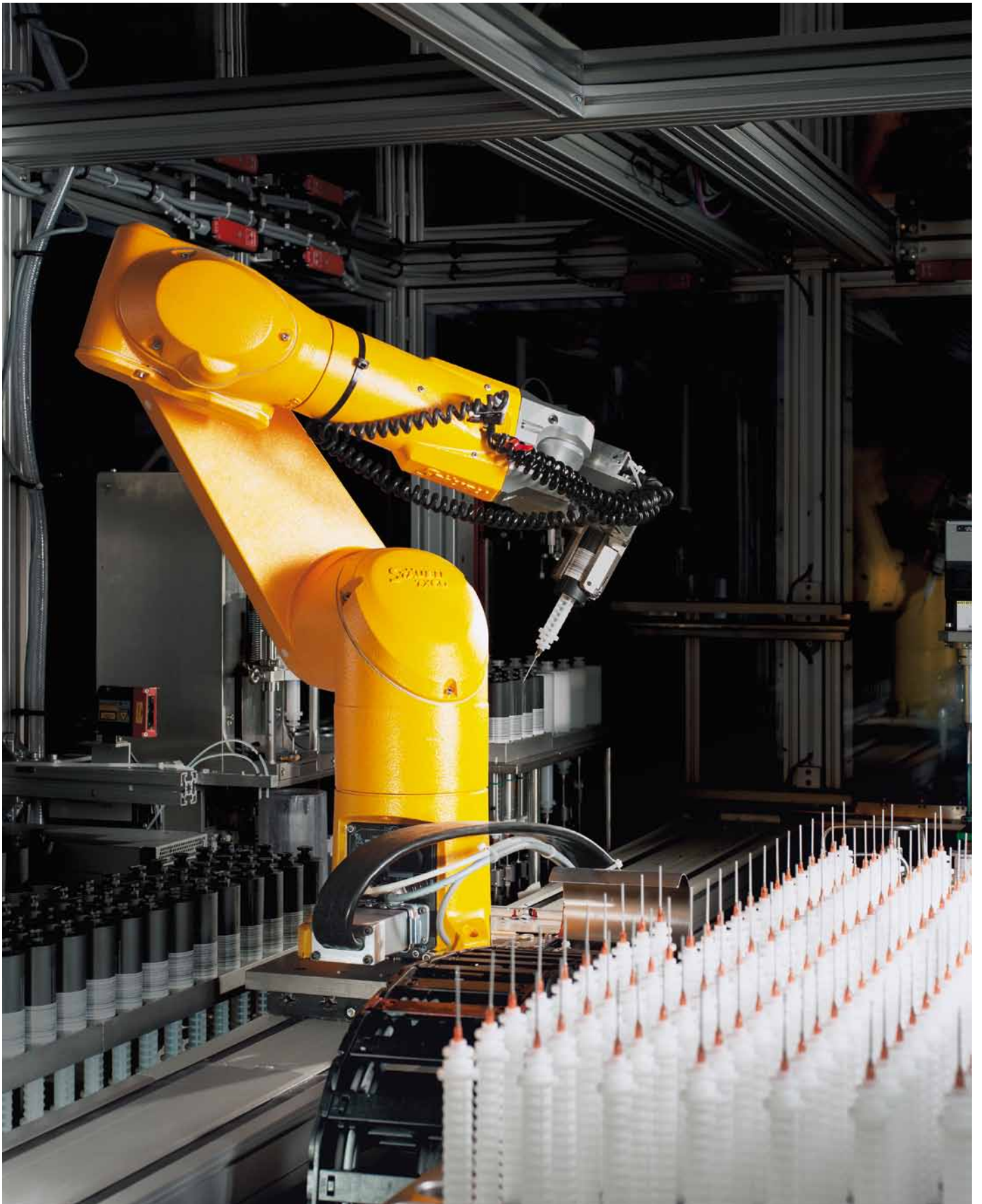
The robot in the combinatorial lab produces up to 140 different paint mixtures in a single night shift.
