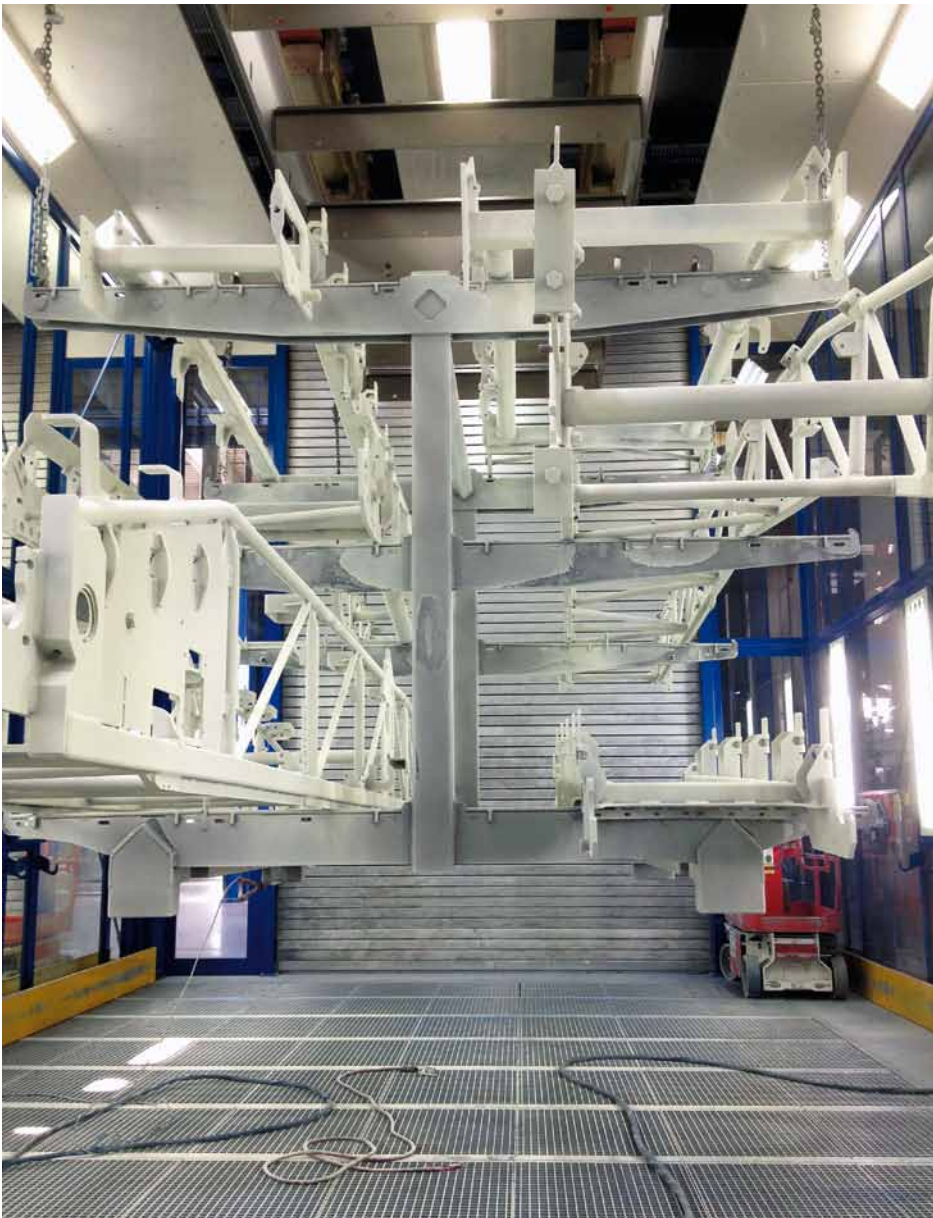
A question of size: A special plant is needed to paint construction machinery.
