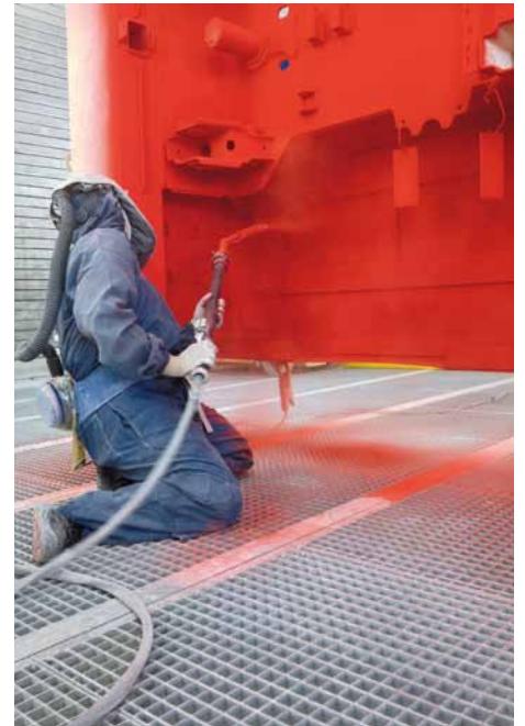
A question of technique: Experts coat construction machinery by hand in a sheath of protective powder paint.
